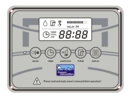
There are one LCD Display, one Indication Light (Red/Green) and five keys in the Dehumidifier touch pad control panel.
