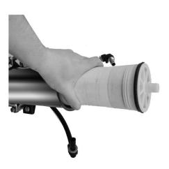
LUBRICATE REPLACEMENT RO AT PERMEATE TUBES BOTH ENDS. REINSTALL RO AND REASSEMBLE HOUSING. BE SURE TO MAINTAIN ORIGINAL PLUMBING CONFIGURATION.
