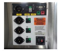
Start/Reset Switch: The START/RESET Switch is used to enable the Compact 20 to produce heat. If at any time power to the control circuit is lost or if a fault condition occurs, the Compact 20 will go into the FAULT/NOT RUNNING mode. Pushing the START/RESET switch will energize the control circuit and restart the Compact 20.
