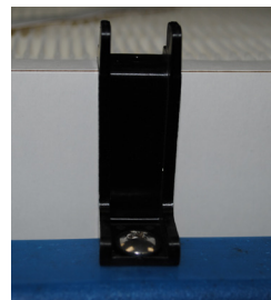
The photo depicts clip in a locked position. Turn counter-clockwise to unlock.
