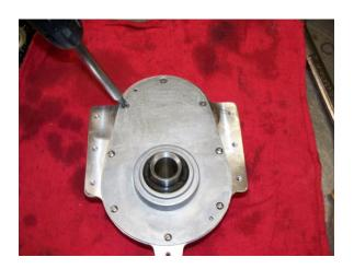
6) Fill Gearbox with 65cc's of 90 weight synthetic gear oil, and use 7/16" wrench to install oil plug P/N: B-009. Check the oil level with a toothpick and there should a ½" of oil at the deepest point.
