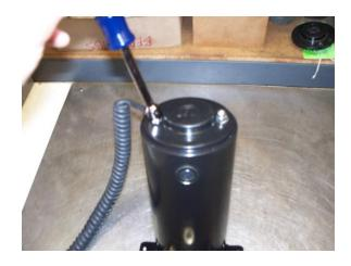
13) Install Carbon Brushes P/N: RP-228, and Carbon Brush Caps P/N: RP-229. Note: Be sure that curvature of carbon brushes matches the rotation of the armature, or premature wear of the carbon brushes may occur.
