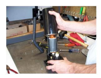
11) Install shim washers P/N: RP-231, spring washer P/N: RP-232, and top bearing P/N: RP-230 (which may be inside motor cap. Install motor cap P/N: RP-201(kit). Note: It is acceptable to install bearing onto armature first, or install motor cap with bearing mounted to cap.
