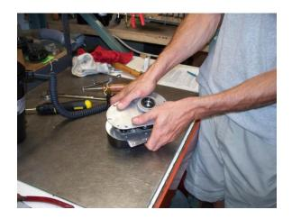
5) Use Phillips Screwdriver to fasten bottom plate screws P/N: S-053, to bottom plate. \*\*IMPORTANT – IF REPAIR IS BEING DONE WITHOUT A VACUUM CHAMBER IT WILL BE NECESSARY TO USE 5 SCREWS WITH NUTS ATTATCHED WHERE THE GEARBOX IS NORMALLY ATTACHED TO THE VACUUM CHAMBER. THIS WILL PREVENT OIL LEAKS WHILE MOTOR IS IN TRANSIT. \*\*
