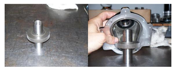
3) Place Upper Gearbox Housing upside down and install Gearbox Spacer P/N: D-2322 (On female shaft) Intermediate Gear P/N: B-2314 (onto Large Dowel Pin P/N: D-043 in center of gearbox), and the O-Ring Oil Seal P/N: O-111 (in groove around outside of gearbox housing). Note: Be sure that the rubber O-Ring stays in its channel during the assembly process.
