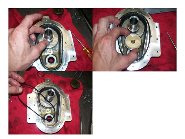
4) Slide Bottom Plate P/N: D-2319 onto Female Shaft. Note: It may be necessary to grease the inside of the large bearing and work the Bottom plate back and forth to walk it down the shaft. \*\* IMPORTANT – BEFORE BOTTOM PLATE IS SEALED DOUBLE CHECK THAT THE O-RING OIL SEAL HAS NOT MOVED OUT OF PLACE, AS THIS MAY CAUSE OIL LEAKS WHEN REPAIR IS COMPLETE.\*\*
