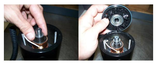
12) Install Motor Mount Washers P/N: RV-457 and Acorn Nuts P/N: S-048, using 3/8" Nut driver, being sure to tighten each side with equal force to ensure a balanced rotation of the armature.
