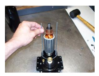
10) Slide Motor Tube P/N: RP-201(kit), down over armature, ensuring that the white field wire is routed on the outside of the all thread motor screws. Note: Be sure
