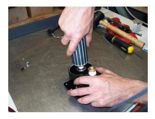
8) Wrap Reducer Bushing P/N: B-010, with Teflon Tape and hand tighten into female shaft. Wearing a heavy glove, grasp Armature firmly and use 7/8" wrench to fully tighten Reducer Bushing.
