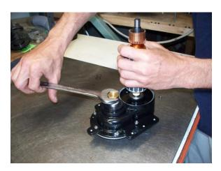
9) Install all-thread motor screws P/N: RV-434, three to four turns.
