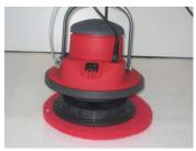
Never leave the machine standing on the polishing, cleaning or micro fibre pad after use. The pads will be squeezed by the one-sided weight of the machine, and smooth working can not be realized anymore. The pad has to be replaced in that case.
