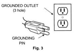
FOR SAFETY: Do not operate machine unless cord is properly grounded.
