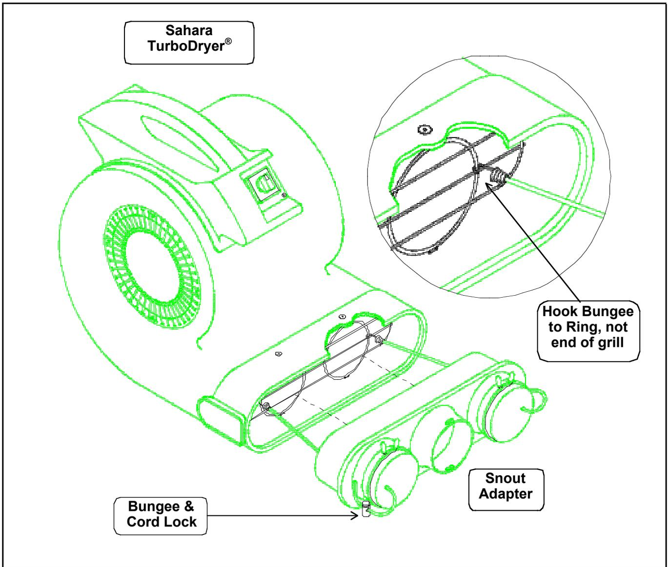
*Clip bungee hooks to the ring portions of the grill. When not using an outlet, cover with vinyl cap and spring clamp.*
