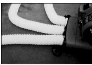
The adapter is made to fit standard 4-inch ducting.
