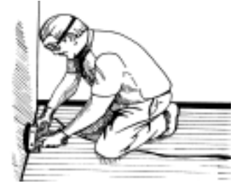
Circular jamb saw used to cut ventilation openings.
