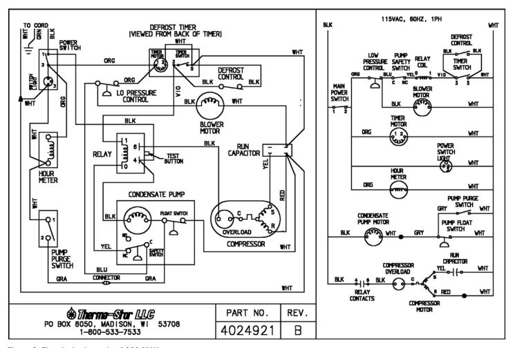
Figure 3: Electrical schematic of 200 MAX
