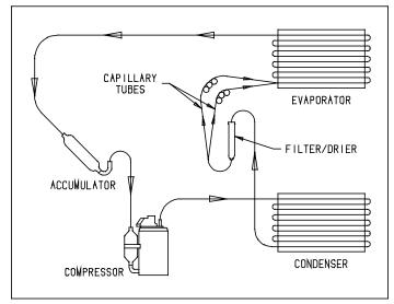
Figure 2: Refrigeration system of Phoenix
