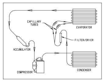
Figure 2: Refrigeration system of Phoenix
