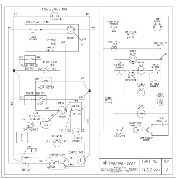
Figure 3: Electrical schematic of Phoenix 300
