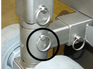
Figure 2: Remove the center hitch pin to steer the Hydro-X during extraction
