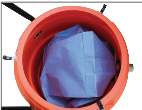
High efficiency 2-ply enclosed, disposable paper filter bag acts as the primary filter to trap and hold dry material for easy handling and disposal. (B524253)
