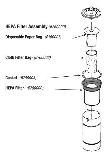
Each Pullman-Holt HEPA filter is tested and certified to provide a minimum efficiency of 99.97% at .3 microns based on IEST-RP-CC001 test requirements.
