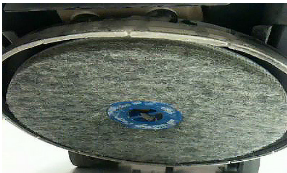
4 Lift and lock deck to inspect burnishing pad for wear
