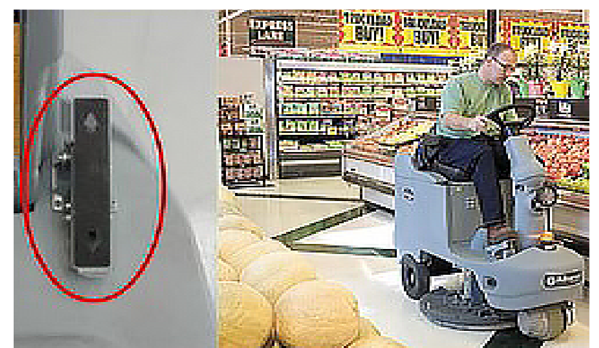
12 Use motion control pedal for forward and reverse. Transport machine to work area
