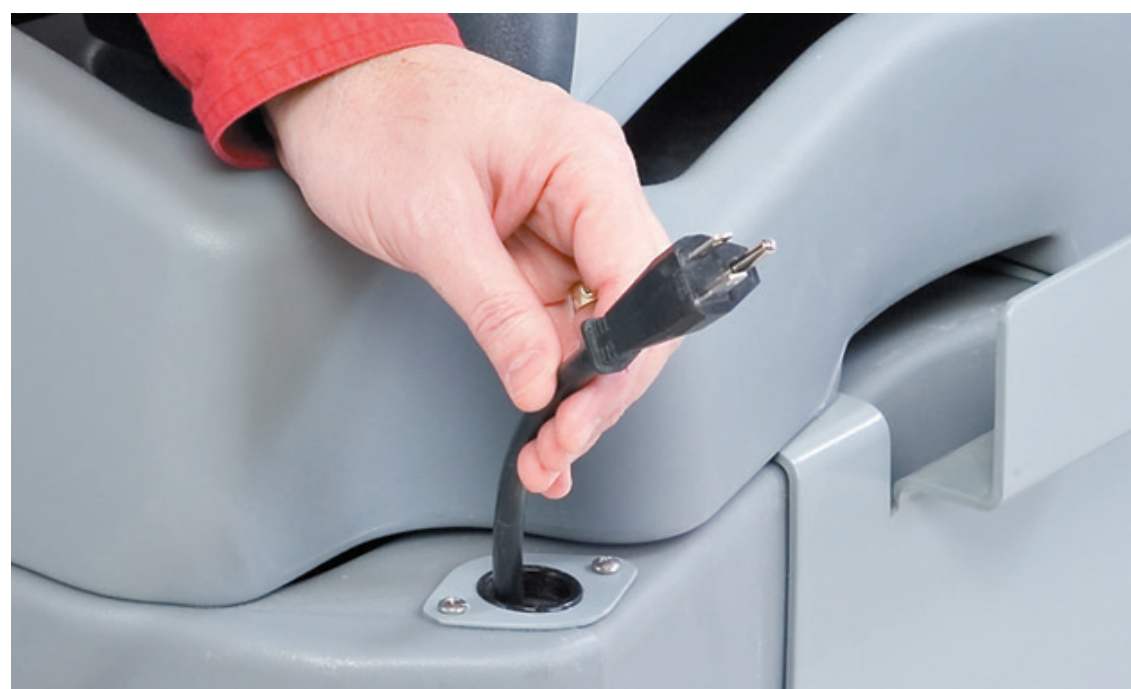
2 Onboard charger: Disconnect battery Store cord inside machine frame
