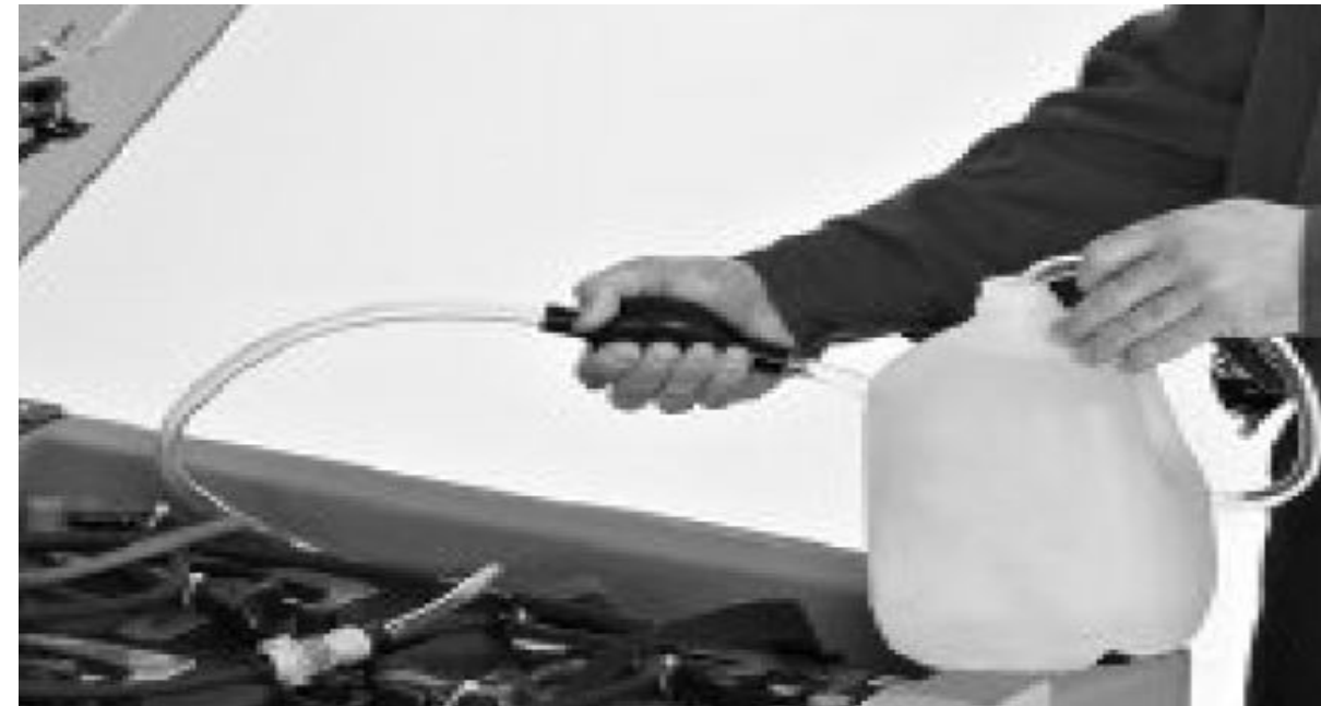
4 Check battery water levels. Optional battery watering kit shown. Check/Replace Pad Shroud Skirt
