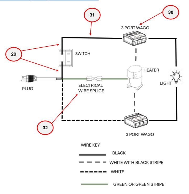
Your Heater is designed to give you years of reliable service. If a problem should arise use the troubleshooting section in the operation manual to diagnose and correct the problem if possible.
