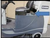
Fill the solution tank 1/3 with water then add appropriate chemical. (Temperature should not exceed 130°F).
