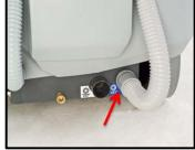
Switch the recovery hose to Wet Pick up connection
