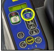
Press the Extract On/Off switch to acknowledge hose change (press again).
