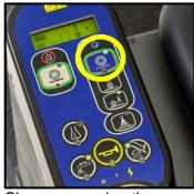
Clean area using the Extract Mode: press Extract On switch (horn will beep).
