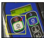
Clean area using Sweep Mode to vacuum debris from the entire area to be cleaned.
