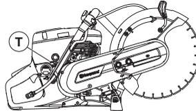
Rec. idle speed: 2700 rpm
