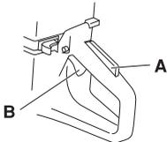
The trigger lock remains pressed in as long as the throttle is pressed. When the grip on the handle is released the throttle trigger and the throttle trigger lock both return to their original positions. This is controlled by two independent return spring systems. This means that the throttle trigger is automatically locked in the idle position.
