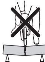
If the blade is pinched or stalled in the kickback zone, the reactive force will push the power cutter up and back towards the user in a rotating motion causing serious or even fatal injury. Be alert for potential movement of the work piece. If the work piece is not properly supported and shifts as you cut, it might pinch the blade and cause a kick back.
