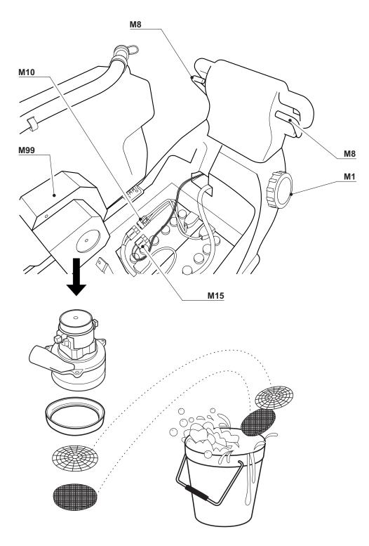
**Recovery tank**: weekly clean it as follows: switch off the machine, switch off the voltage, open the dirty water tank. Remove the suction motor cover M99 (page 9). Then remove the suction motor: the filter and the net will be cleaned underneath. Drain the dirty water from the M2 (page 7) pipe. Remove the dirt that has settled in the tank. To do this, open the cap M0 (page 7) to have visibility inside the tank.
