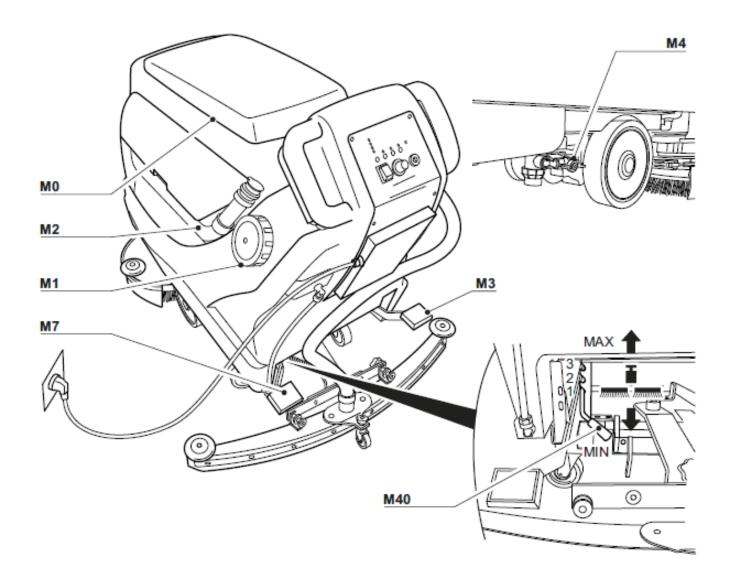
Turn the key switch to position ON (I). In this position the machine can already move backward and forward as described below. Next press butt  $O_1$  (control panel) then button (brush). At this point the water dosage and vacuum will start automatically. If desired, they can be switched off individuall *mu*ith (wate *L* d (vacuum ) buttons.
