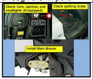
Inspect controls, parking brake and install main broom. Fill dust guard system with clean water (optional for machines with this feature)
