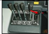
Set the throttle (engine models only). Parking brake should be off
