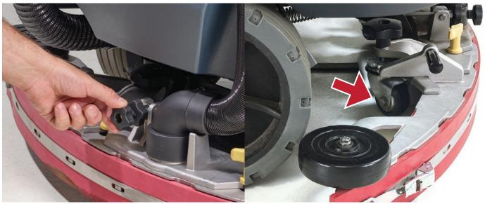
7. As necessary adjust the tilt angle of squeegee so blade has uniform contact tip to tip. Verify squeegee casters rotate and pivot freely and are in contact with the floor when squeegee is in the down position.
