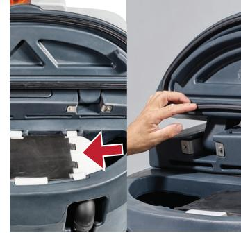
**4.** Empty debris basket. Recovery tank seal cover must be correctly installed, clean and in good condition. Check for gasket wear.
