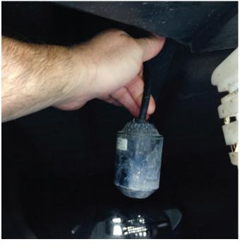
**2.** Inspect recovery tank float switch operation.
