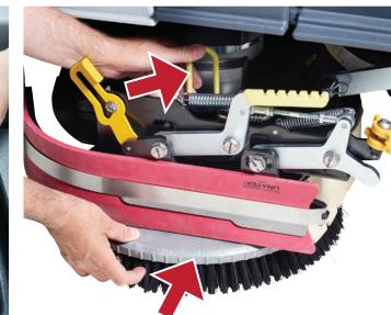
12. Install brushes by positioning against guides. Press brush install button.
