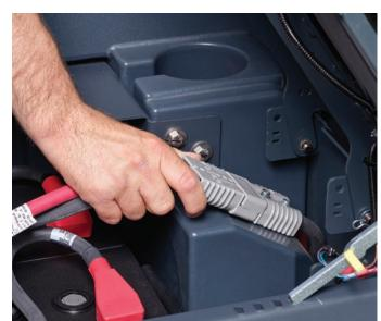
3. Check that battery cables are connected.
