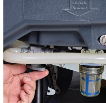
**2.** Verify the solution valve is open and aligned with inlet and outlet ports of valve.
