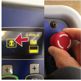
2. E-stop icon appears on display when E-stop switch is engaged.
