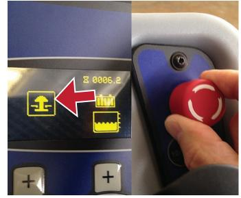
2. E-stop icon appears on display when E-stop switch is engaged. Twist E-stop switch to enable machine function.
