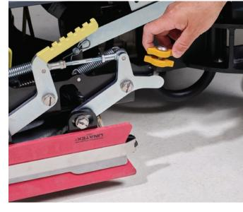
13. Adjust side skirt heights and inspect blades for wear or damage.
