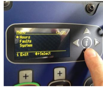
18. Press "i" scroll down to faults and press ">" button to view faults.
