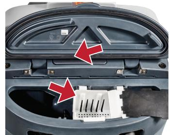
4. Recovery tank seal cover must be correctly installed and in good condition. Clean and empty debris tray.
