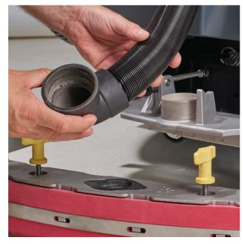
**1.** Check if the suction hose is properly installed, not plugged, or cracked/torn.
