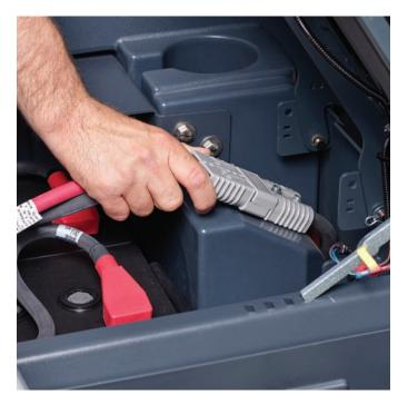
**3.** Check battery cables are connected.
