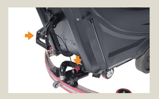
Use the handle to lower or raise the squeegee to the floor. Adjust the squeegee angle with the knob to adjust suction performance if needed.
