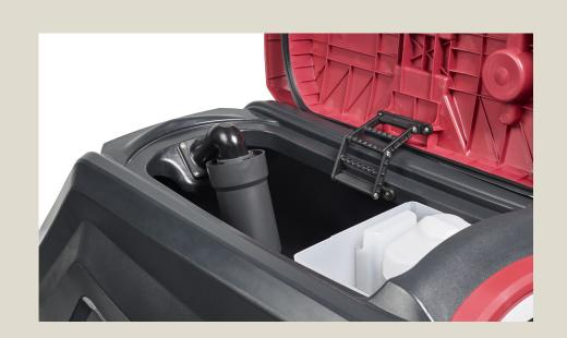
**Daily:** Inspect and rinse the float ball cage. Inspect, check and clean the debris tray and clean the lid gasket if required.
