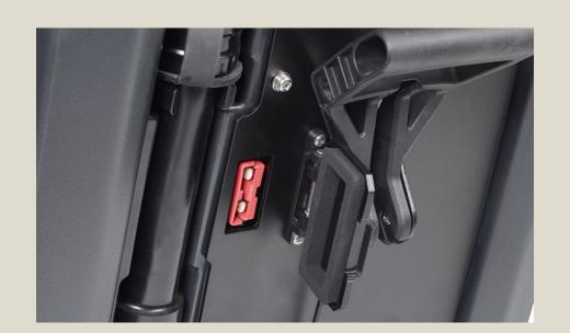
Daily: to charge the battery, connect the charger connector to the machines outer charging connection, and connect the charger to the wall socket. Check the charger indication light so the charging have started. If the machine is supplied with On-board charger, tip the recovery tank and connect the on-board charger in the same way.
