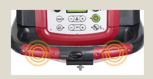
Place the machine in working mode and press any of the two red safety switches to activate the machine.
