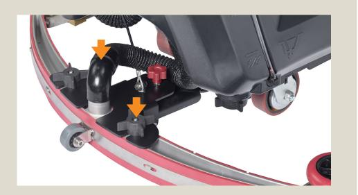
Install the squeegee using the thumb nuts. Attach squeegee hose.
