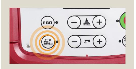
Floor Preparation Button (orbital) for stripping: pad pressure will be set up to maximum, solution flow will be set to minimum, machine speed will be held at 1 km/h 0.6miles/hour
