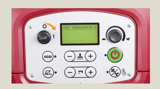
Turn on the key and verify there is enough battery power to complete the work.
