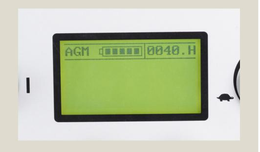
**Daily:** if the battery indicator is low, put the machine on charge. Battery should be on charge if empty, not in use or if not being used for coming 8-10 hours.
