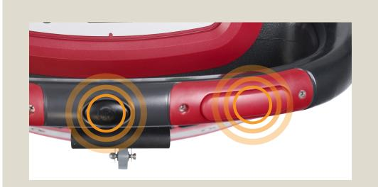
Pressing either of the red safety switches and the black reverse button together will put the machine into reverse.
