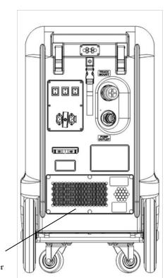
**HEPA exhaust filter grill.** Thumbscrews allow easy filter replacement. To order
