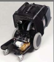
Several models are available, including 150, 200 and 500 PSI pumps, dual 2-stage or 3-stage vacuum motors and optional internal heaters, (see opposite side).
