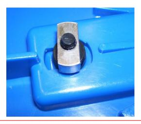
Retaining Nut Aligned to Secure Inner Shell
