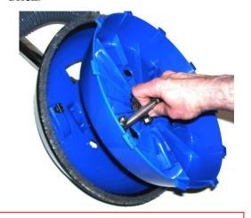
Separate the Outer & Inner Shells
