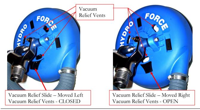
Using the SX-15 with extractors with higher air flow will generally require the vacuum relief vents to be opened more. Using the SX-15 with smaller portable extractors may require the vacuum relief vents to be closed for the best water recovery. When using the Hard Boot the vacuum relief vents will usually be opened more than it is when using the Brush Ring with the same extractor.
