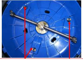
Three Rectangular Retaining Nuts
