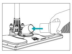
**1.** Connect vacuum hose from a portable or truck-mounted extractor. 2" cuffs will slide over the vacuum port and 1.5" cuffs will slide inside.
