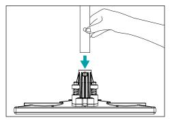
**1.** Press in the spring button and slide the handle into the handle base. Make sure the spring button lines up with the hole. It will snap into place. **NOTE:** The handle may fit tightly on the first installation but it will loosen up over time.
