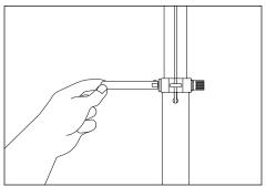
lock lever outward to loosen the clamp. Slide the handle up to desired height and press the lever back inward to tighten.
