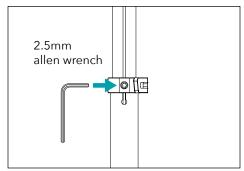
2. With the handle in place, pull the cam **OPTIONAL:** To permanently lock handle location, tighten set screw until it pierces inner handle tube.
