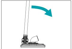
**5.** When you are ready to move to a new position, pull the handle back to release suction. Move the SOS PRO to a position that is directly adjacent to, but not overlapping, the previous extraction position.
