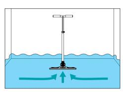
**3.** If there is standing water, place the SOS PRO in the center of the room to remove the standing water down to the carpet lev-
