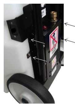
Insert 4 - #10-32 x 1-1/4" long Stainless Steel Machine Screws through the holes on the Handle with the Basket facing toward the rear of the unit.
