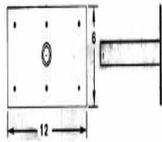
(WM) The wall mount bracket is available for the convenient installation of reel to wall or door of van. The reel still can be equipped to operate live.
